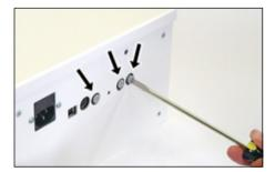
4 Use the flathead screwdriver to remove the three fuses. Make a quarter turn counterclockwise.
